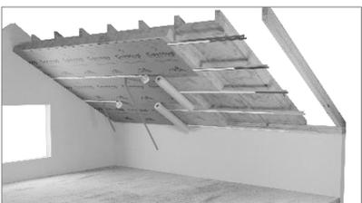
2. Further vapour control layer strips should be installed with a suitable overlap, which is printed on the membrane and bonded with single-sided (e.g. Corotop FIX) or double-sided tape (e.g. Corotop MIX).
